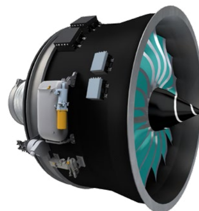
More Electric Engine concept reproduced with permission of Rolls-Royce plc
